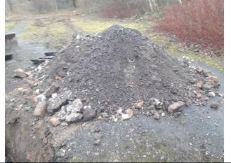
Trial Pit 130 Remarks: 1.Terminate due to rapid groundwater strike at 2.0 m bgl.
