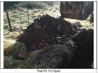
Remarks: 1.Terminated at 2.00m bgl due to collapse. 2.Rapid groundwater strike at 1.80m bgl. 3.Excavation slow due to cobbles within Made Ground. 4. Large concrete and brick obstructions within strata at 0.40m and 0.30m bgl. Stability: Unstable
