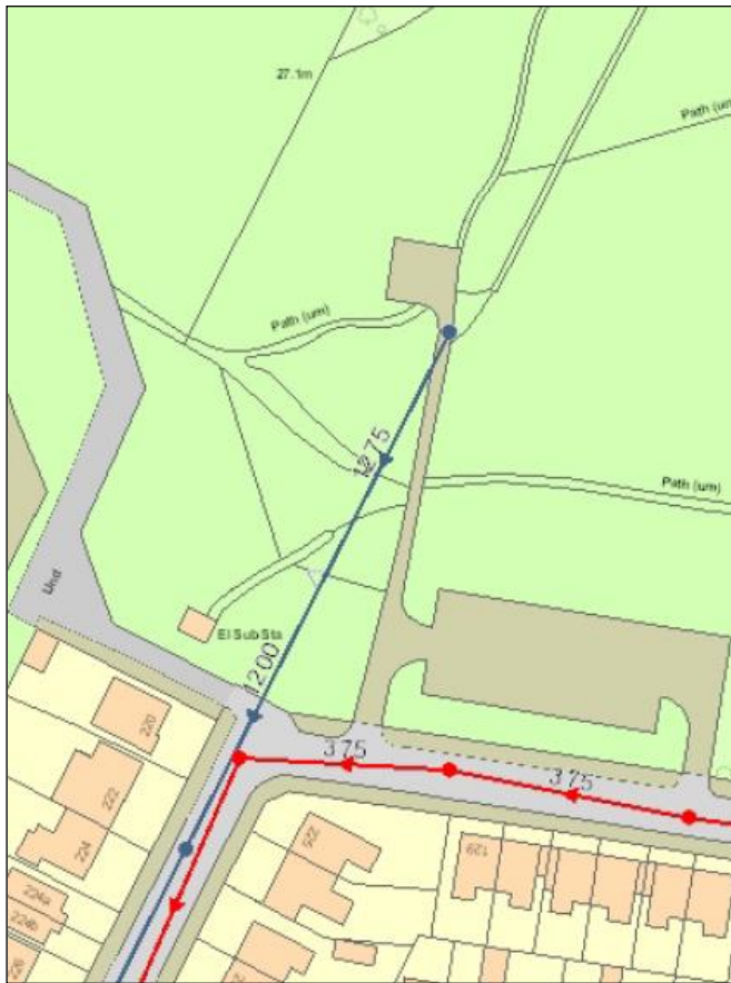
Figure 2.5.3 United Utilities surface water 1275m dia pipe from manhole near old sports pavilion
