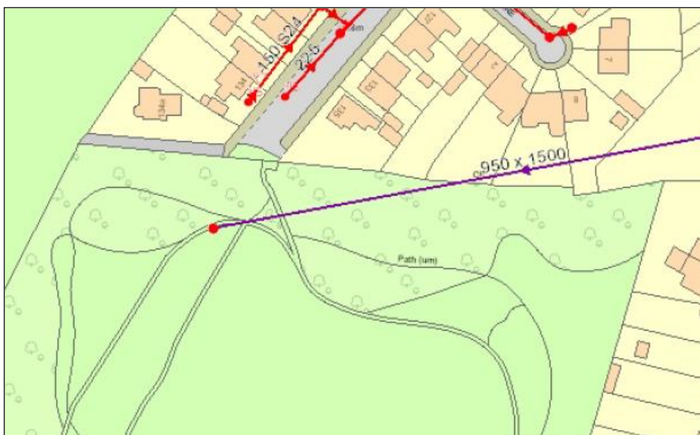
Figure 2.5.4 United Utilities discharge overflow 950 x 1500 pipe to manhole within the North development plot.
